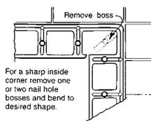
For a sharp inside corner remove one or two nail hole bosses and bend to desired shape.
