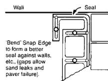
Bend Snap Edge to form a better seal against walls, etc., (gaps allow sand leaks and paver failure).
